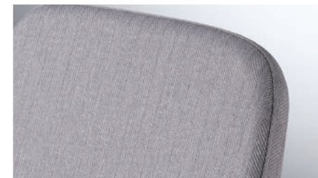
Fabrics: A sewing gusset was finished with a single stitch.
